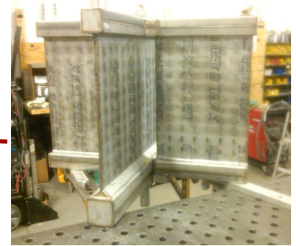
Internal Fuel Pre-Heater
