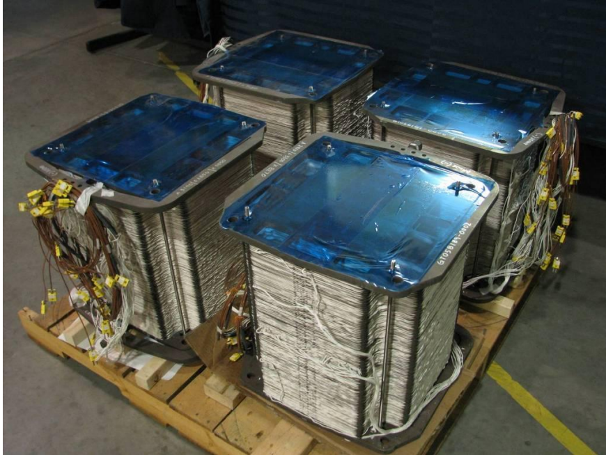
4x 96-cell stacks to be integrated in a 60 kW module as shown on a shipping crate
